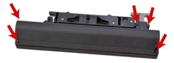
Remove five TORX10 screws holding the top cover and take off the lid.
