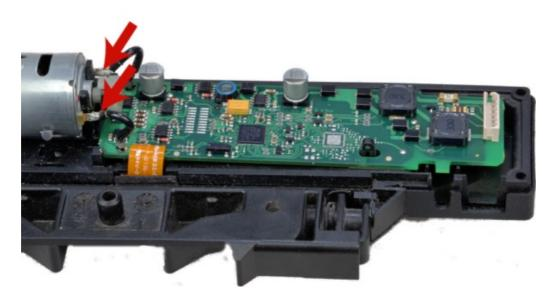
Unsolder the wires from electric motor.
