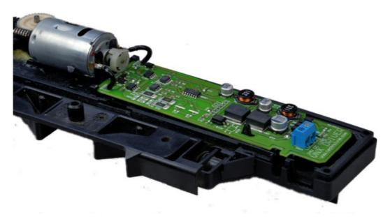
Install a VNX-A controller & solder the wires to the electric motor only (do not resolder the orange flat ribbon cable as it is to be extracted). Module is ready for operation. Connect the supply wires and assemble back the lid.
