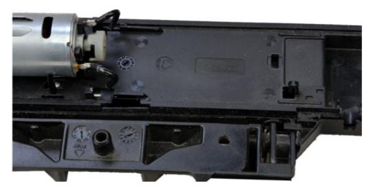
Disassembled module is ready for installation of VNX-A controller.
