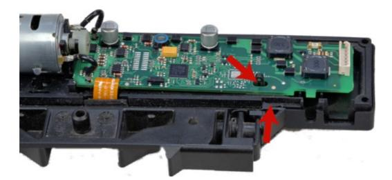
Remove the electronic module by pressing shown plastic snaps.
