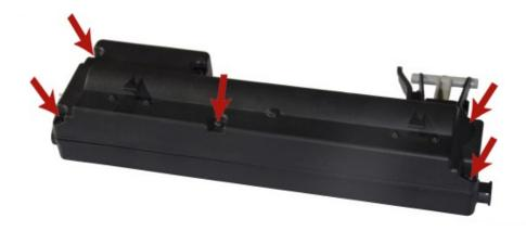
Remove the five TORX10 screws holding the top cover. Remove the cover.
