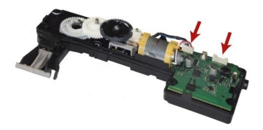
Disconnect the plugs from an electronic module.
